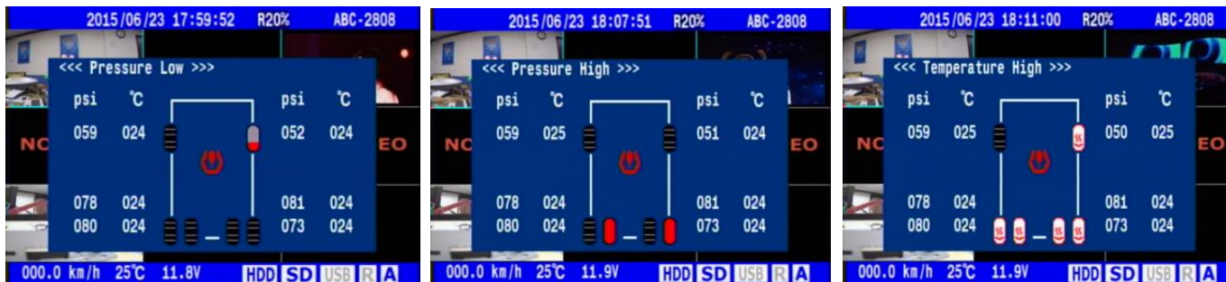
Low pressure Alarm
